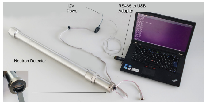
Figure 1: The detector is a plug and play solution with a self-contained control unit. Multiple detectors can be connected to large arrays.
