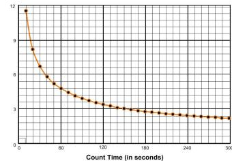
Confidence of Detection 90% (1.3 sigma) False Alarm Rate 1/100 (2.33 sigma) 25 micro R background Eff. - 9.7%
