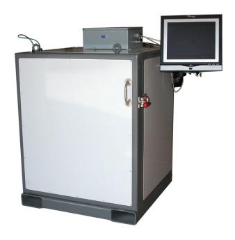
THE TSA BM286 IS DESIGNED TO SCREEN ITEMS UP TO AND INCLUDING 55 GALLON DRUMS WEIGHING UP TO 1,000 LBS FOR RADIOACTIVE CONTAMINATION AND IS IDEAL FOR MONITORING PRIOR TO RELEASE FROM THE FACILITY.
