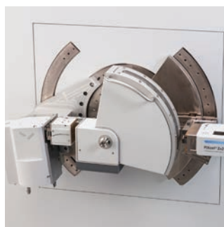
Attachment for SAXS/WAXS measurements with evacuated beam path (patented). For highly dilute and low-contrast samples and for increased data collection speed.
