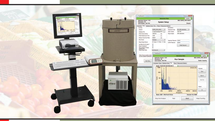
"Complete, out-of-the-box solution designed specifically for measuring gamma ray emitting radioactive contaminants in food and water."
