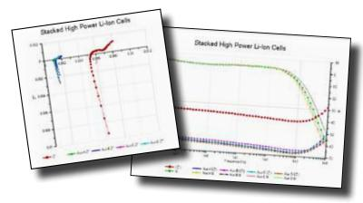
These example low-noise measurements are taken from a stack of Lilon cells, and show the impedance of the overall stack and of individual cells in the stack.
