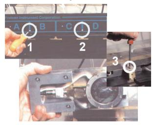
Any MDS detector and window can be accessed by removing 2 front panel screws and 1 internal screw.
