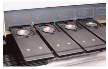
Repeatable counting geometry is assured using the removable sample carriers that adapt to different depths of planchets. Independent position sensors prevent erroneous data due to a partially closed drawer.
