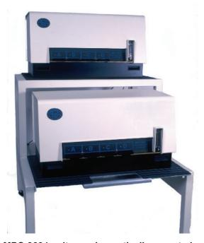
Two MPC-9604 units can be vertically mounted on the optional MDS-RACK shown above. If maintenance is necessary the lower unit is easily pulled forward for cover removal (as pictured). Squeeze the handle to release the brakes and the lower MPC-9604 glides forward on its roller bearing supported plate. Release the handle and the brakes engage. The heavy duty rack distributes the weight to reduce floor loading.
