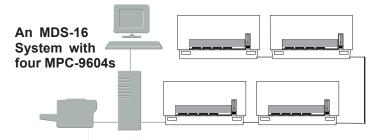
Communications between the PC and the MPC-9604 units is fast, reliable, and inexpensive utilizing IEEE RS-485 standards and Protean's exclusive PICNET II protocol. The control software automatically identifies new additions and configures itself to match.
