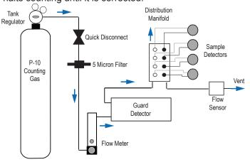
Each MPC 9604 includes a self-contained gas distribution and flow monitoring system ready to connect to a regulated supply of P-10 gas (nominally 10 lbs/ln²).
