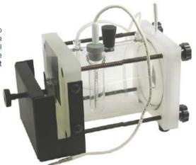
The practical design of the Model K0235 Flat Cell makes it simple and easy to use for corrosion and/or coatings research. It can accommodate a wide range of electrode sizes, eliminating the need for machining or special mechanical procedures. It disassembles quickly and easily, operates with a 250 mL sample volume and simplifies electrochemical corrosion measurements.
