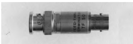
TF50 Feedthrough terminator, 50 \Omega , BNC. Provides 50- \Omega ( \pm 2\% ) 1-W feedthrough termination of 50- \Omega cable at high-impedance inputs.
