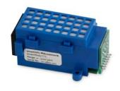
Infrared gas sensor using dual beam technology, with measurement and reference channel, for monitoring room air and process control applications. Integrated evaluation electronics for drift and temperature compensation.
