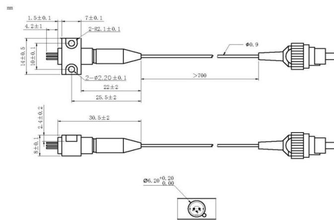
**8-Pin Package View (built-in TEC) :**
