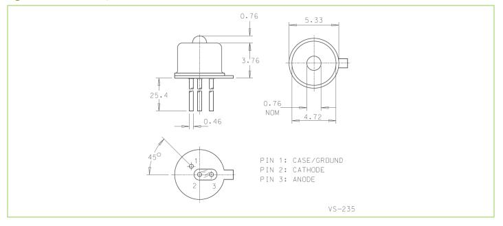
Figure 15-C30902SH-TC/-DTC, TO-66 with flange outline, reference dimensions shown in mm (inches)
