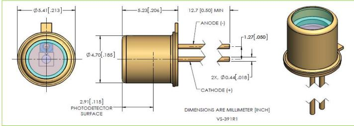
Figure 14 – C30902BH, reference dimensions shown in mm
