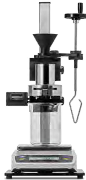
Flow through an orifice — with cylinder
