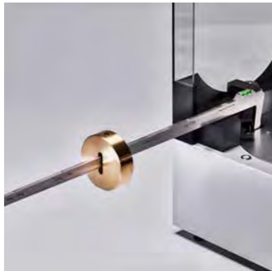
Static qualification with a single SmartCal™ reference weight that can be applied in multiple positions
