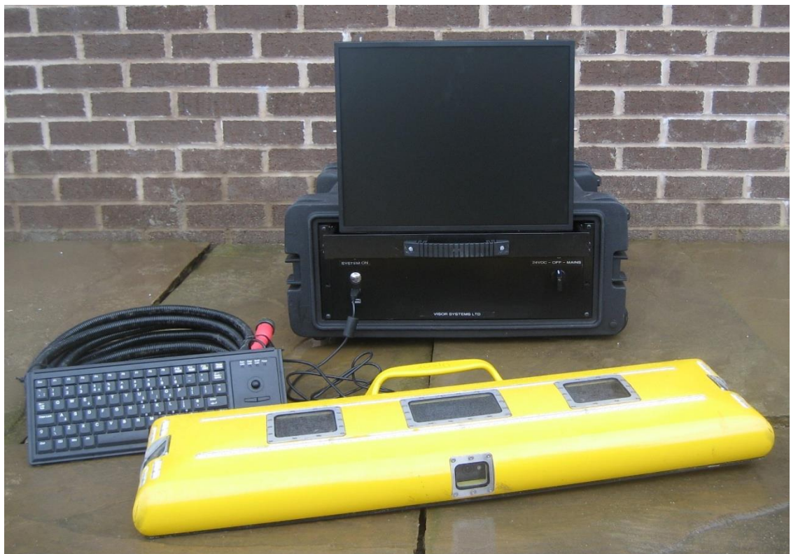
Visor Portable UVIS System Control Unit (VCU) & Optional Detail / Zoom View Monitor
