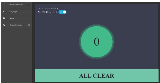
LaserWarn's user interface can provide operators with a simple Green/Red Go/No Go dashboard for instantaneous situational awareness. Should a higher level of detail be required, real-time spectra from gases and threats can be displayed. If a multi-threat scenario occurs, LaserWarn can identify multiple gases simultaneously.
