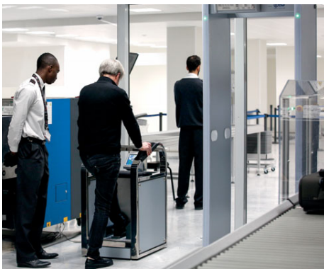
Passenger Screening by Walk-Through Metal Detector (WTMD), Shoe Scanner (SAMDEX) and passenger body control through PAT-DOWN
