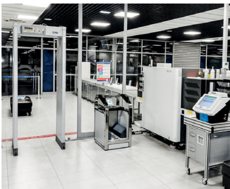
Passenger Screening by Walk-Through Metal Detector (WTMD), Shoe Scanner (SAMDEX) and passenger body control through Explosive Trace Detector (ETD)
